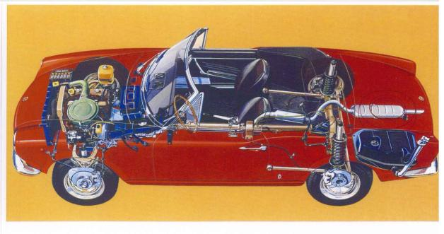
An open sports two-seater powered by a twin overhead camshaft, 96 hp engine, providing ample power and zestful acceleration. 5-speed all-synchromesh gearbox. Suspension designed for fast driving, plus servo-assisted brakes. Brilliant and safe; a car with a sporting character and yet built with an eye for comfort all the same.
